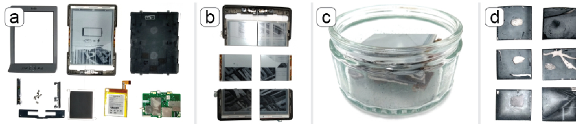
Fig. 2. The extraction process developed within FabricatINK in order to gain access to E ink for exploration and adoption as a material for use within personal fabrication.
