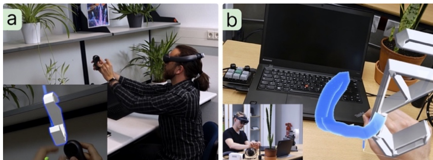
Figure 1: In our prior works, we explored how 3D-printing may be supported through in-situ search and remixing of objects from a model repository (e.g., Thingiverse). Mix&Match (a) lets users preview designs in their future context and remix them [7]. ShapeFindAR (b) allows users to search for designs to 3D-print through rough sketches, vague keywords, and iterations with results [8].
